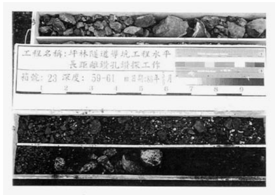
Photo-2 Fractured rock samples from the second borehole at depth 59-61 m.
